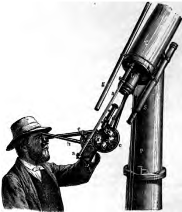
FIG. 84.—The spectroscope attached to the telescope for solar work. P, pillar of telescope; T, telescope; S, finder; L, eye-end of telescope; A, B, supports of spectroscope; C, collimator; D, prism-plate; E, observing telescope; H, micrometer.
